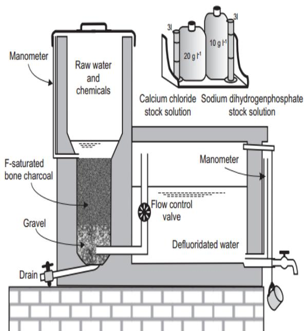
Figure 2: Schematic of Contact Precipitation of Fluoride in Ngurtodo<sup>5</sup>
