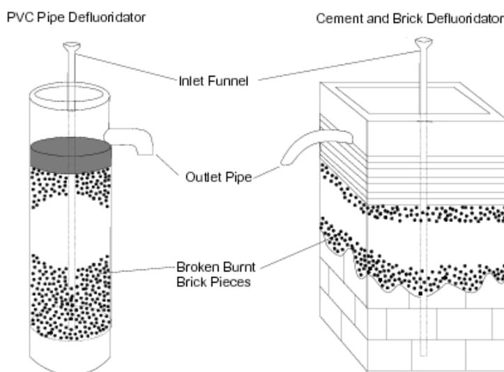
*Figure 1. Design of the clay and soil defluoridation unit used in Sri Lanka*
