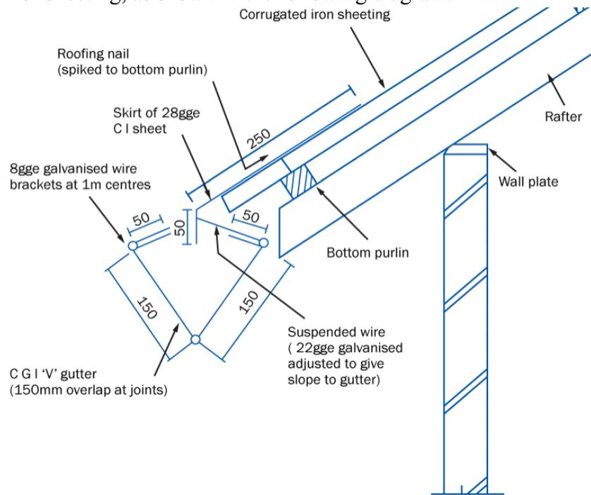
Figure 9: Section of Typical Roof Guttering
