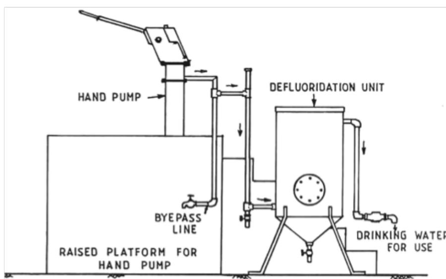
*Figure 6: A hand-pump attached defluoridation unit*
