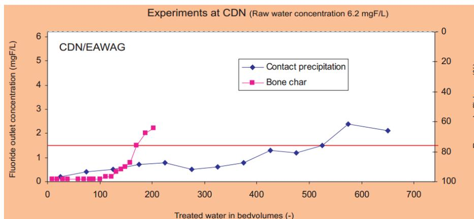
Figure 4<sup>10</sup> : Experimental Testing Comparing Contact Precipitation and Bone Char Techniques
