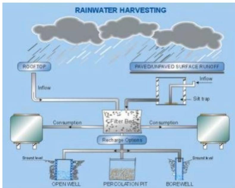
*Figure 10: Schematic of Rainwater Harvesting and Storage System Options*
